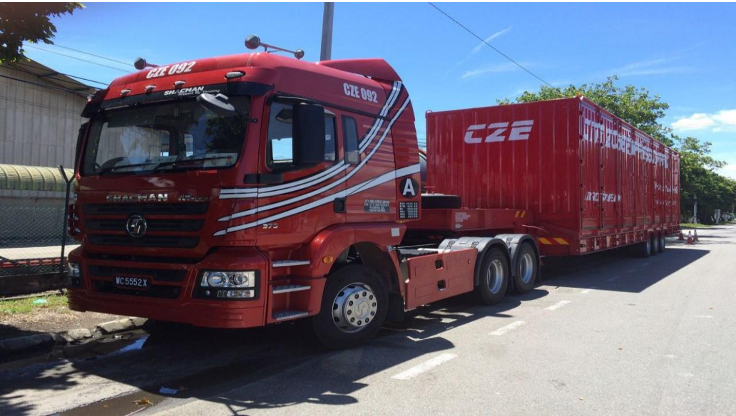
*Low Loader with Customised Container Cabin (14.0 L x 3.0 W x 3.20 H M)
